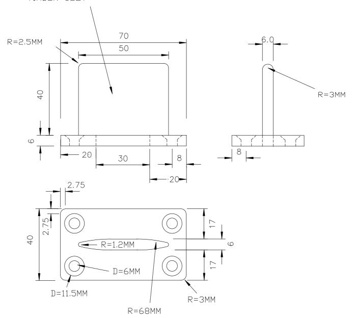
STAINLESS STEEL FLOOR GUIDE FOR TIMBER DOORS WELDING TO BE GROUND AND POLISHED AS GUIDES ARE VISIBLE
