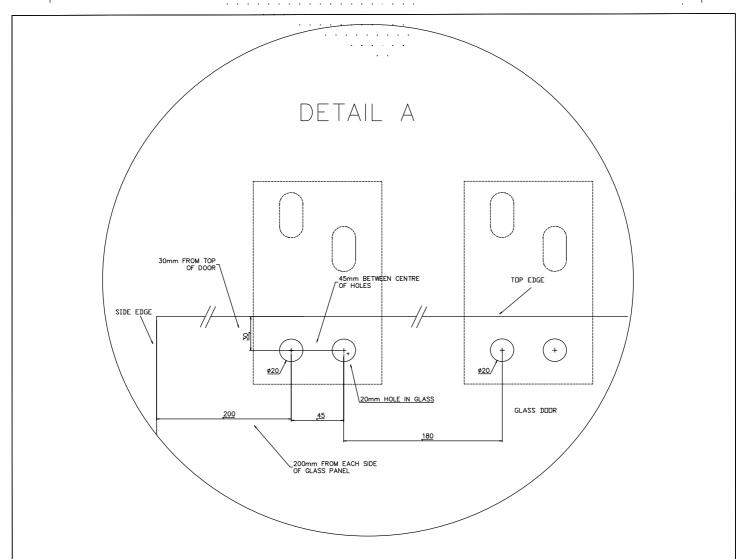
FRAMELESS DOOR PANELS OVER 1800mm WIDTH, HOLES FOR PATCH FITTINGS
